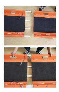
**4.** After install the basket stretcher, there should no crevice between the two parts.
